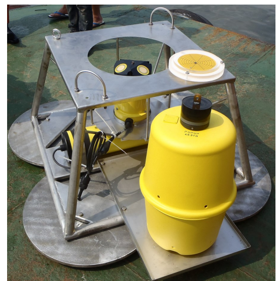
The Pentair COASTAL-HM fitted with real time wave measurement, current profiling and meteorological instruments assisting navigation in Straits of Singapore
